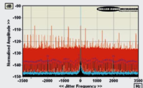
**ABOVE:** 48kHz/24-bit jitter spectra from a Chord Mojo over USB (red, via standard PC; black, via Roon Nucleus+; cyan, via Melco N1ZS20/2 USB player out)
