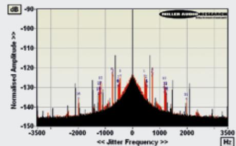
**ABOVE:** 48kHz/24-bit jitter spectra from an OPPO Sonica DAC over USB (black, via Melco N1ZS20/2 USB player out; red, via Roon Nucleus+ with markers)
